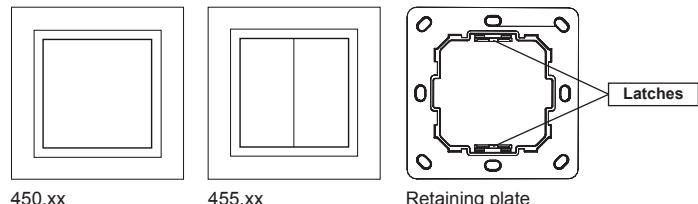
The Easyfit wall transmitter is a universal, extremely flat standard switch element that can be integrated into numerous control programmes by different manufacturers. The universal element is compatible with the switch programs listed in the table. Frame integration is similar to universal inserts for antenna sockets.
