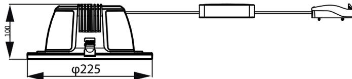
Cut-out hole diameter - Ø200mm
