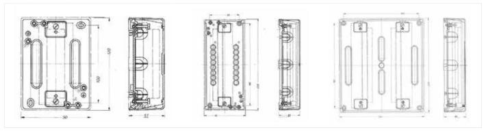
Disclaimer: Max. permittable depth of built-in parts 38 mm
